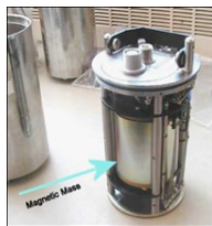
Seismometer w/cover removed
