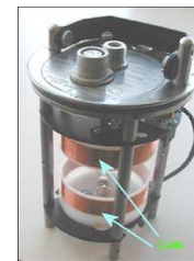
Seismometer w/magnetic mass & cover removed
