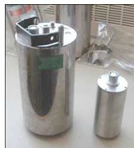
Seismometer w/magnetic mass removed
